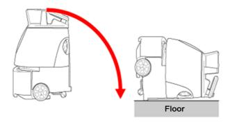
■ Please check that the secondary battery power button on the bottom of the machine is off (⇒see "Secondary Battery Power Button") . Also, remove the protective film on the cliff sensor.
