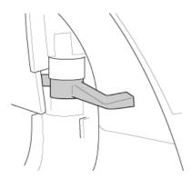
Insert the catches at the bottom of the cover in the bottom of the dustbin (1), and close the cover while holding the dustbin access handle down (2)
