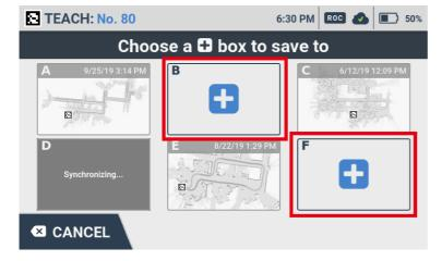
Once the number of saved routes has reached the limit, either delete existing cleaning routes (⇒see "Deleting Cleaning Routes"), or scan a different Home Location Code.
