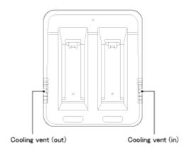
■ Check visually for anything abnormal (discoloration, corrosion) and for any abnormal sound, etc. from inside the charger
