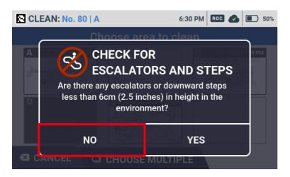
• Tap "YES" and a barrier warning screen appears. Check the warning message and tap "CONFIRM". Tap "CANCEL" and a cautionary screen of autonomous cleaning appears.
