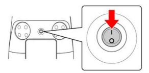
■ Home screen will be displayed when the Power button is turned On. Do not turn the power Off until the Home screen is displayed.
