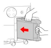
4 Check that the battery is locked
