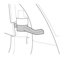
Insert the catches at the bottom of the cover in the bottom of the dustbin ① and close the cover while pushing down on the dustbin access handle ②
