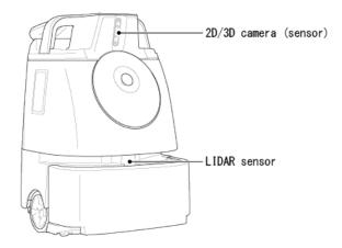
2 Check that nothing is caught in the gaps around the bumper, and that the machine moves back several centimeters when the bumper is pushed slightly
